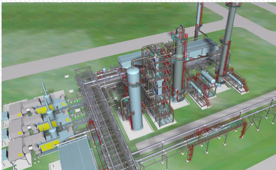
Model tridimensional instalatie de fractionare gaze
