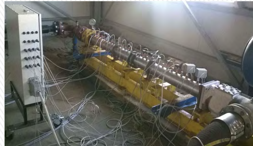
Multiphase pump equipped with pressure and temperature sensors
