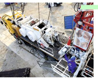
The main parts of the workover unit are assembled on a frame mounted on the chassis:
