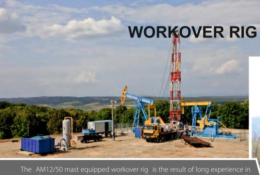
The AM12/50 mast equipped workover rig is the result of long experience in manufacturing (AM 10) and repairing of workover rigs. It is designed for intervention and overhaul of oil and gas wells without derricks, of which working depth is in accordance with 50tf hook loads, to perform the following tasks:
