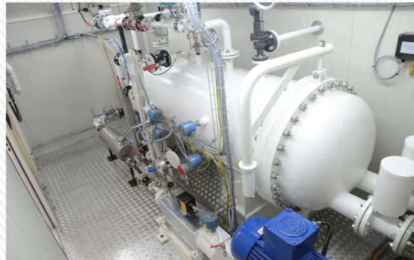
Bi-phase calibration separator
