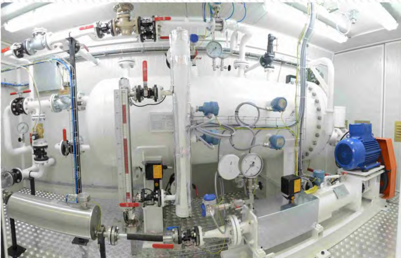
Bi-phase calibration separator
